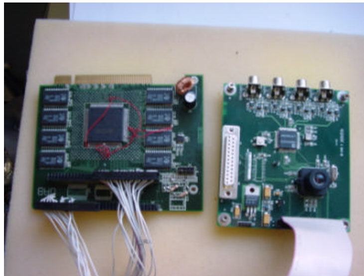
Fig 3. RIC (left) and sensor (right) prototyping boards used to prototype image acquisition.
